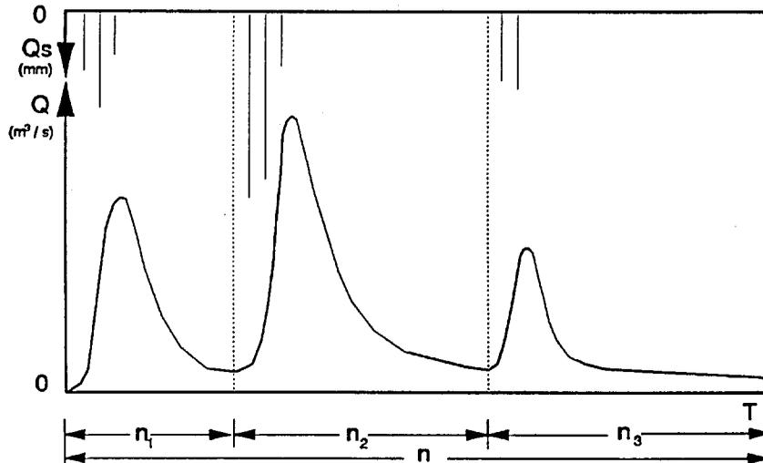
Figure 2. The example of flood events, where  $Q$  is the observed discharge,  $Q_s$  is the calculated runoff or net precipitation,  $n$  is the number of time steps in the whole calibration period. In this example, the period is split into three subperiods; the time steps are  $n_1$ ,  $n_2$  and  $n_3$ . In each subperiod,  $Q_s$  corresponds to its flood event
