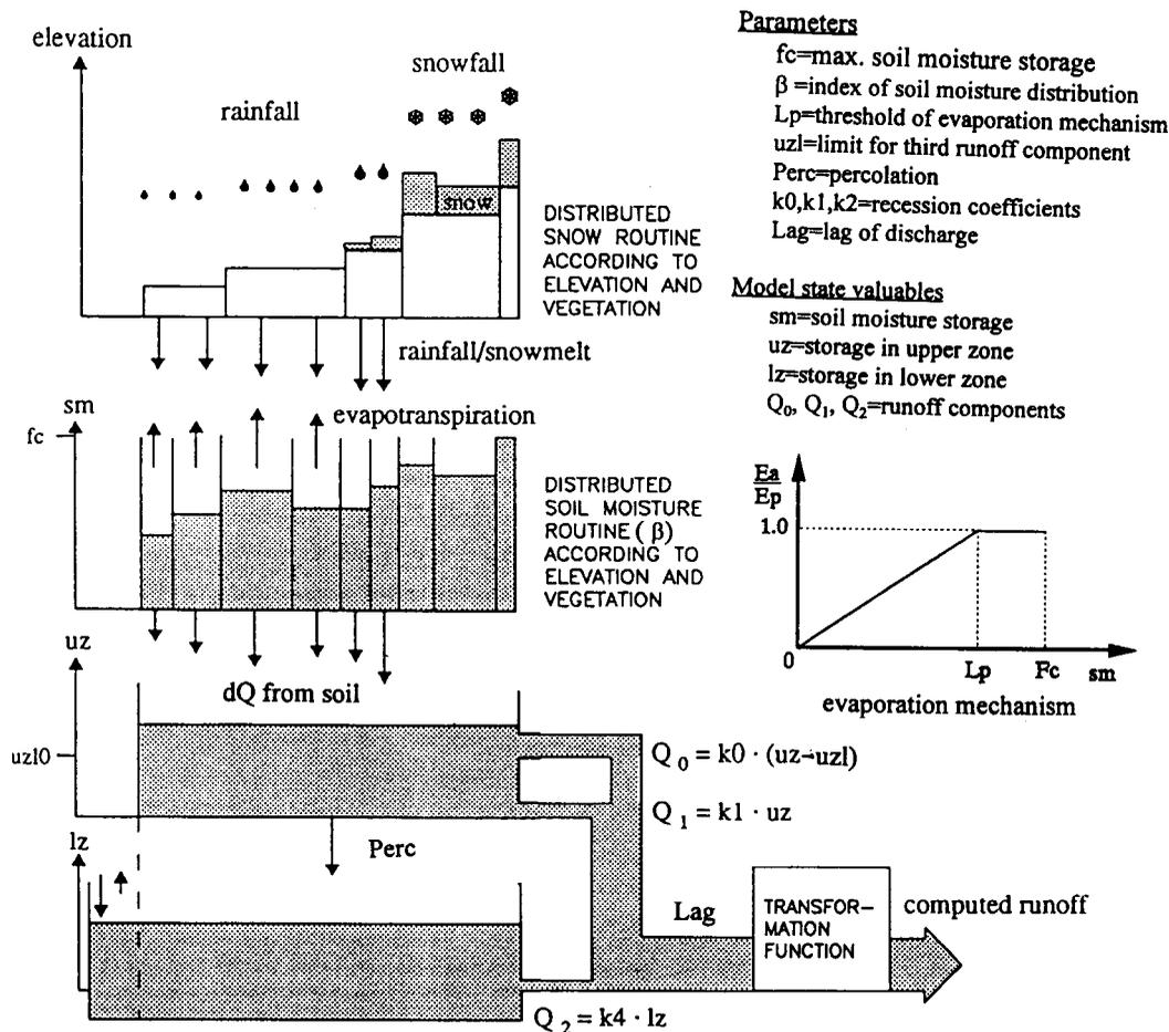
Figure 1. The general structure of the HBV model as applied to one sub-basin
