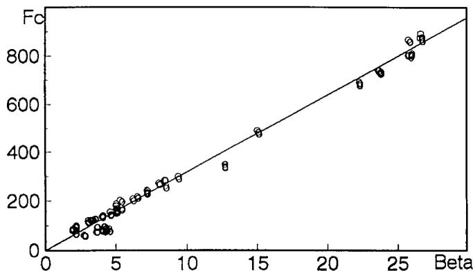
Figure 3. The relationship of the optimum values of  $Fc$  and  $\beta$  for the tests. The values were derived from different tests, including different parameter combinations with the different objective functions and initial values. There are about 60 points in the figure in total.  $Fc$  in mm
